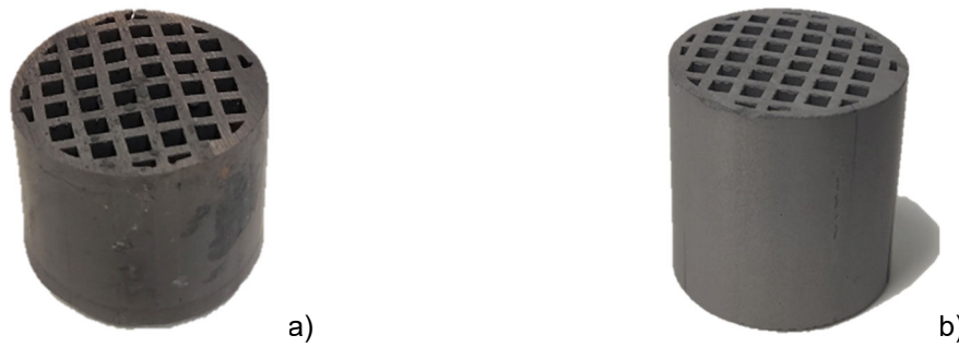
Figure 5: Photographs of extruded structures with the 44 cpsi die after calcination at 1300°C: a) CMO and b) Sr-doped CMO, i.e. CS10MO honeycombs.
