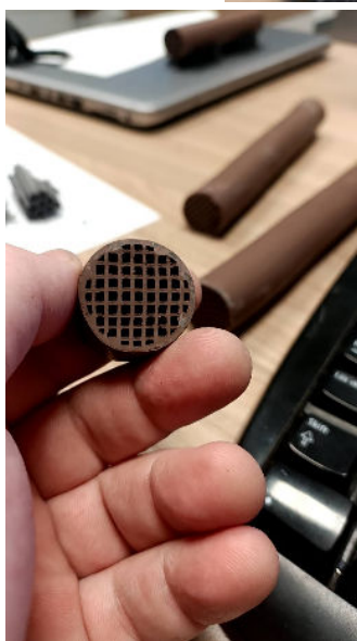
Figure 4: Green bodies from the preliminary scald-up extrusion tests at LET. The pictures present extruded segments from a \varnothing 25 mm die for the preparation of flow-through membranes at LET
